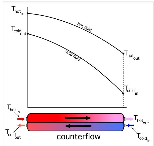
Figure 5-6 show how the temperature of the two liquid streams would change as they flow through a heat exchanger piped for parallel flow versus one piped for counterflow.
