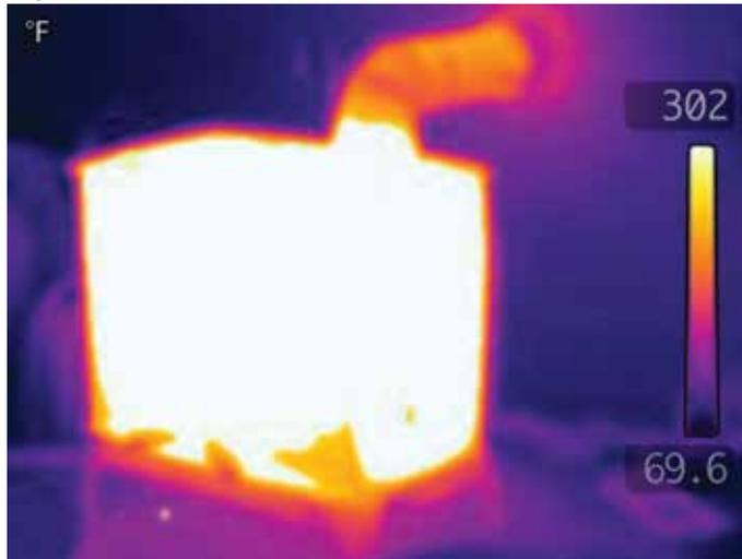
The thermal radiation coming from the wood stove is captured by the imaging system in a special camera and converted to visible colors. The correspondence between these colors and the surface temperatures is shown on the scale at the right of the image. This image shows that the sides and top of the stove are hot (around 300°F), while some of the materials behind the stove are at a normal room temperature of about 70°F.
