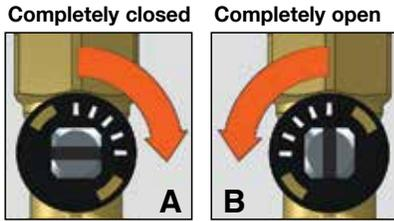
For the flanged version, rotate the adjusting handwheel 90° for the complete opening and closing of the valve as shown in (A) and (B). When at the desired position, lock the adjustment screw.
