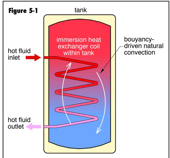
This heat exchanger geometry is commonly used for indirect domestic water heaters that heat cold domestic water in the tank by passing hot water from a boiler or other heat source through the immersion coil.
