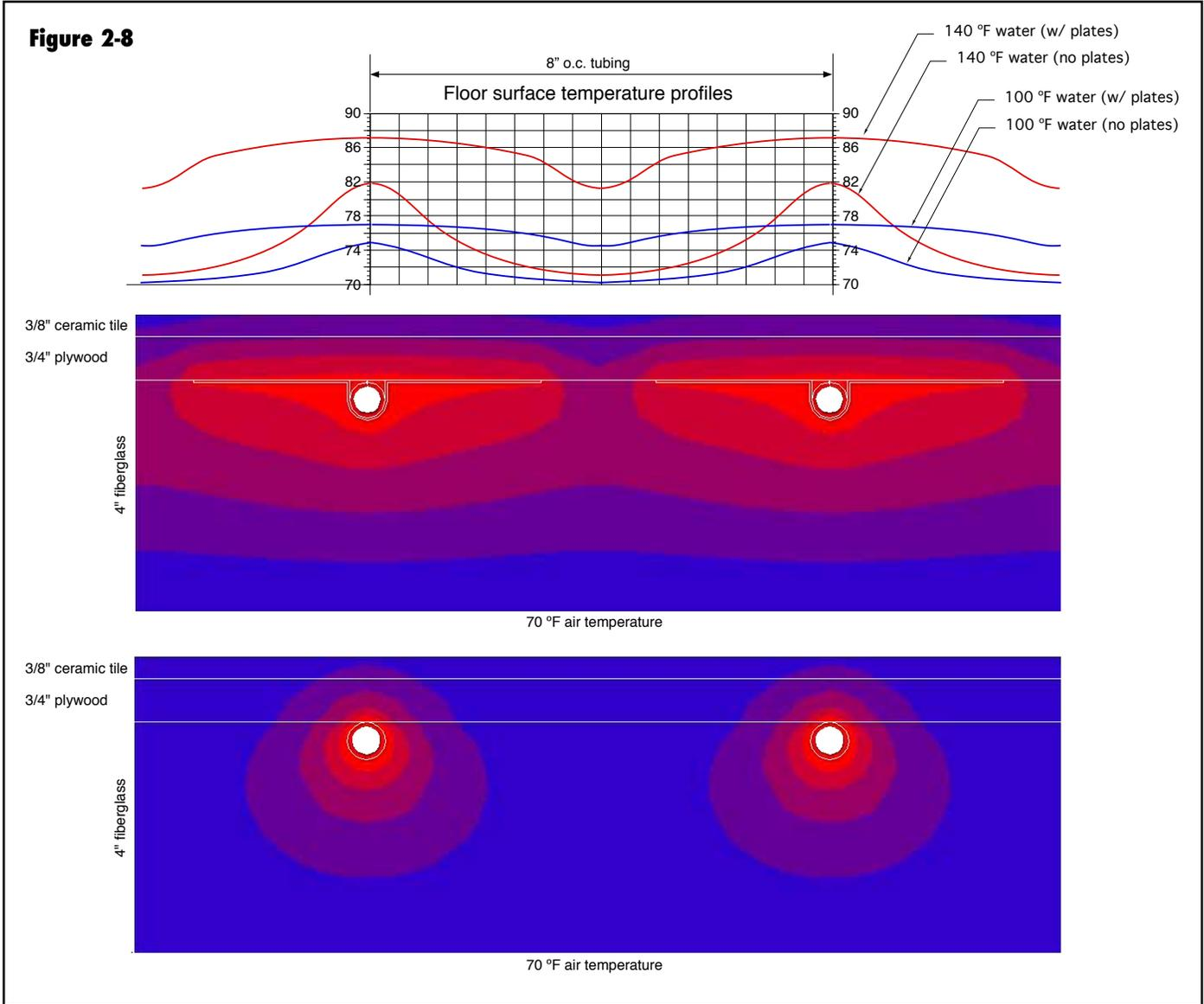
only variable between the two models is the presence of 6-inch-wide by 0.024-in.-thick pre-formed aluminum heat transfer plates in the upper graphic, and the absence of any plates in the lower graphic.
