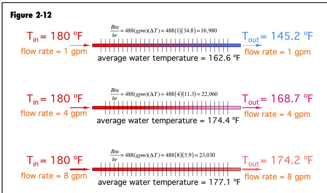
The heat output rate increases rapidly at low flow rates. It continues to increase as flow rate increases, but the *rate of increase* is much slower at higher flows.
