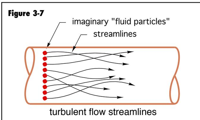
The erratically shaped streamlines present during turbulent flow create good mixing. A small quantity of fluid that's close to the tube wall one instant could be swept into the bulk of the fluid stream the next instant. This decreases the boundary layer thickness, and significantly improves convective heat transfer.
