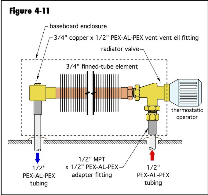
90° turn as it passes through the valve, and flows into the baseboard element. The other end of the finned-tube element can be equipped with a transition adapter (straight or 90°) to convert from 3/4" copper to 1/2" PEX or PEX-AL-PEX.
