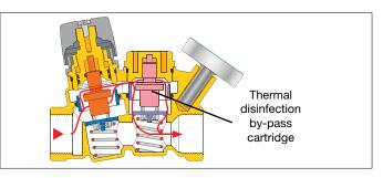
Alternately, the 1163 series models incorporate a by-pass valve for thermal disinfection which is activated by a optional field mounted thermo-electric actuator, code 656 series, controlled by an automation system.
