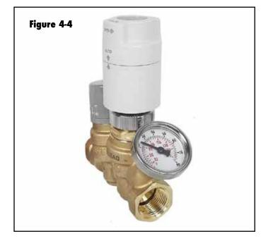
The ThermoSetter<sup>™</sup> balancing valves could also be equipped with temperature sensors, rather than dial thermometers, to provide a building automation system with temperatures at the return of each recirculation riser group. Those temperatures could be recorded to verify successful completion of each thermal disinfection cycle, based on maintaining the return end of each riser group at a specific temperature for a specific minimum time.
