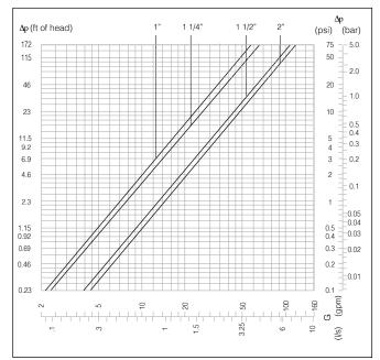
Flow should never exceed standards for pipe size and material.
