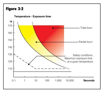
While it may seem intuitive to never set the temperature controls that regulate domestic water heating above a maximum safe temperature, such as 110°F, there are circumstances where this is not possible.
