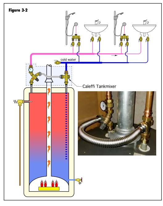
In this system, which does have downstream not devices to further reduce temperature, water the outlet temperature from the thermostatic mixing valve would typically not be set above 120°F. Even lower outlet temperature settings such as 110°F may be required in some circumstances.
