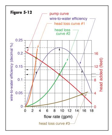
to-water efficiency occurs at a flow rate that is close to the center of the pump curve. For this particular circulator, it occurs at a flow rate of about 9.3 gpm. Ideally, the intersection of the pump curve and the circuit's head loss curve will be at or near this point.
