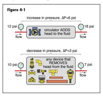
Using pressure gauges to detect changes in the head of a liquid is like using thermometers to detect changes in the thermal energy content of that liquid.
