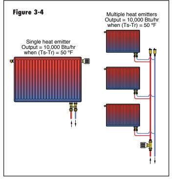
heat emitter(s) will release 10,000 Btu/hr into the building. If the supply water temperature is only 25°F above the room's air temperature, the heat emitter releases 5,000 Btu/hr into the building.
