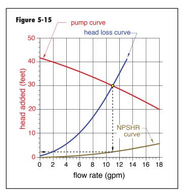
Avoiding cavitation is simply a matter of ensuring the piping circuit's NPSHA exceeds the NPSHR of the circulator under all possible operating conditions.
