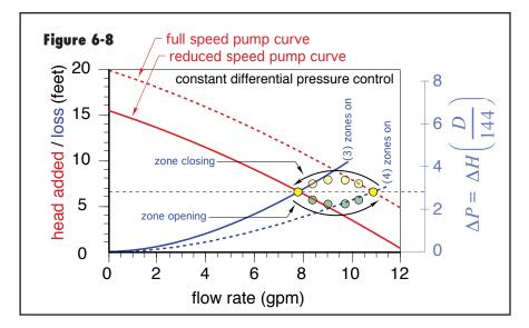
differential pressure, and begin to slow the circulator's motor. This causes the pump curve to move downward, and thus the yellow dots representing the progression of the operating point do the same. Within 5 or 6 seconds, the operating point settles to the intersection of the new head loss curve (shown in solid blue) and the reduced speed pump curve (shown in solid red).
