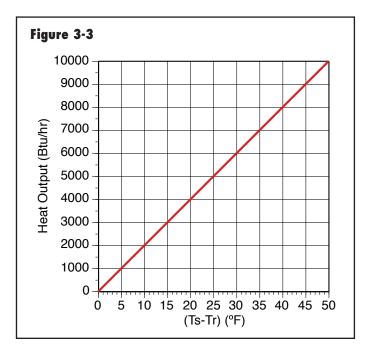
This graph might represent the heat output of a single heat emitter, such as a panel radiator, or it could represent the total heat output of a group of the same heat emitters that are all supplied by a parallel piping distribution system, as shown in Figure 3-4.
