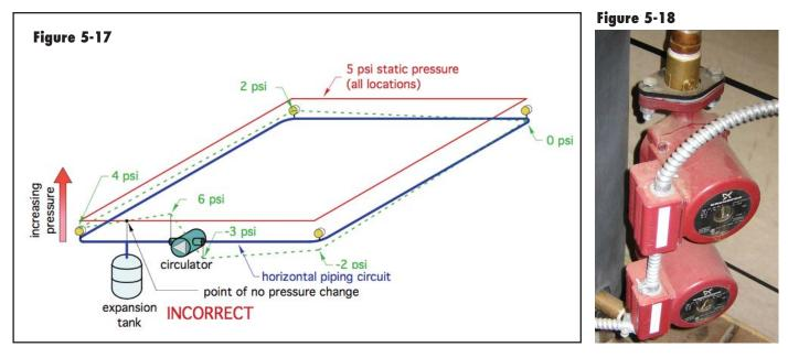
change) remains at 5 psi. The resulting dynamic pressure profile is shown in Figure 5-17.
