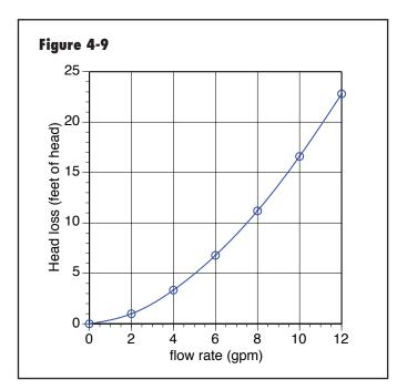
is an essential step in properly selecting a circulator for that circuit.
