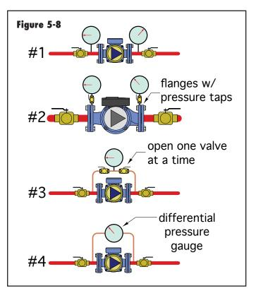
Configuration #1 shows two pressure gauges mounted into the piping just upstream and downstream of the circulator. The differential pressure is the pressure on the discharge side of the circulator minus the pressure on the intake side. This method requires accurate pressure gauges in both locations, since any error in either gauge will affect the differential pressure value.
