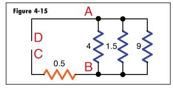
To find the overall hydraulic resistance of the circuit, start by combining the three parallel hydraulic resistances into a single equivalent hydraulic resistance using Formula 4-6. This requires use of a calculator that can work with exponents. Any scientific calculator, including those in smart phones, can be used for this calculation.
