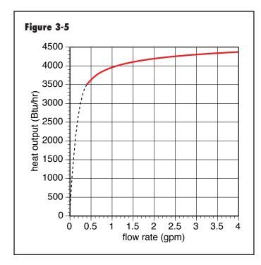
tube baseboard being supplied with 160°F water. The baseboard this graph is based on, is rated to release 600 Btu/hr per foot of element length when the element contains 200°F water moving at a flow rate of 1 gpm.
