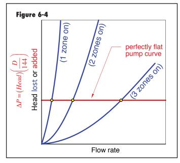
pressure as zone valves open and close. This change is undesirable because it causes an increase in flow rate through zone circuits that remain on whenever other zones close, and vice versa.
