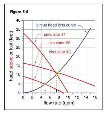
Notice that even though the curves for circulators 1 and 2 are quite different, they intersect the circuit's head loss curve at almost the same point. Therefore, these two circulators would yield very similar flow rates of about 7.5 gpm and 7.8 gpm in this circuit. The flow rate produced by circulator 3, about 5 gpm, is considerably lower.
