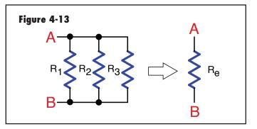
The equivalent resistance of a group of parallel hydraulic resistances represents the same hydraulic characteristics as the original parallel resistances. A given circulator
