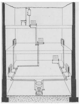
Notice that the piping is either vertical or slightly sloped. This encourages buoyancy-driven flow and helps prevent air pockets from forming within the piping. Such pockets could block flow.
