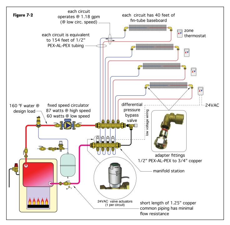
$$n_{d} = \frac{Q_{delivered}}{w_{e}} = \frac{(4 \times 11,221)\frac{Btu}{hr}}{(87)watt} = 516\frac{Btu / hr}{watt}$$
