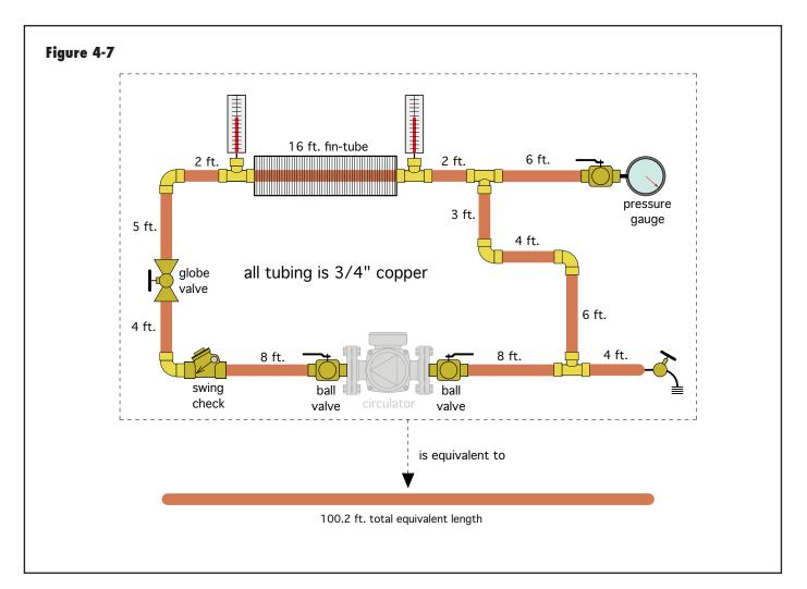
Example: Determine the head loss of the circuit shown in Figure 4-7, assuming it has 140°F water flowing through it at 5 gpm.
