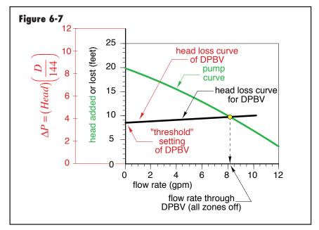
condition. A properly sized DPBV can now be selected based on the manufacturer's maximum recommend flow rate for a given valve size.
