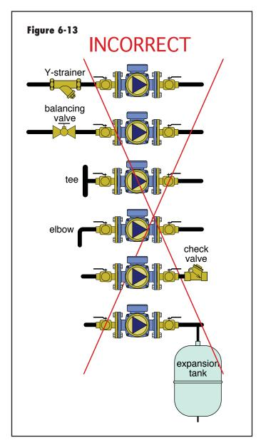
Under the right conditions, this could lead to circulator cavitation (see Figure 6-13).
