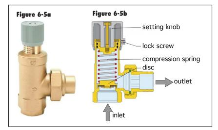
seat to compensate. This allows increased flow through the valve with minimal variation in the differential pressure between the inlet and outlet ports.
