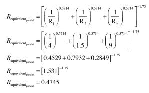
Notice that the equivalent resistance is smaller than the smallest of the individual branch resistances. *This will always be true*, and is therefore one way to check that the calculations are done correctly.
