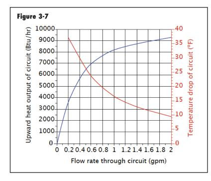
This behavior is not limited to fin-tube baseboard. It also applies to other heat emitters such as fan-coils and radiant panel circuits. Figure 3-7 shows what happens with upward heat output and temperature drop for a 300-foot long circuit of1/2" PEX tubing, buried in a bare 4-inch thick concrete slab at tube spacing of 12 inches. The circuit is supplied with water at 110°F. The room temperature above the floor is 70°F.
