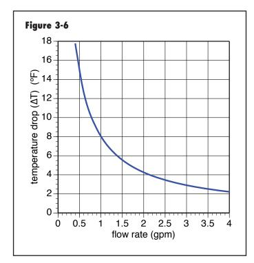
At 4 gpm, the temperature drop across this baseboard is only about 2.2°F. At 2 gpm, it's about 4.2°F, and at 1 gpm, the  $\Delta T$  is about 8°F. If the flow gets down to 0.4 gpm, the  $\Delta T$  is just under 18°F. The temperature drop along the baseboard naturally changes as the flow rate through the baseboard changes. The notion that any heat emitter "wants to," or even *can*, remain at a fixed temperature drop as the flow rate changes is not supported by these results.
