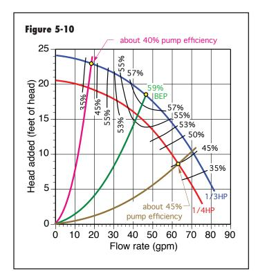
The green head loss curve in Figure 5-10 intersects the blue pump curve at the BEP, and thus the pump, with the 1/3 HP motor, operating in a circuit with this head loss curve, would be operating at its highest possible pump efficiency of 59%.
