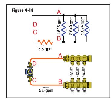
As a check, add up the branch flow rates. Their total should equal, or be very close to, the flow rate in the common piping. In this case, the branch flow rates add up to 5.499 gpm, which is very close to 5.5 gpm. The slight difference is due to rounding off the numbers for the branch flow rates.
