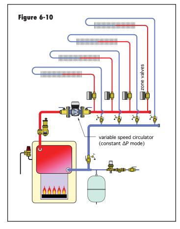
This is quickly sensed by the electronics in the circulator, and they respond by increasing the motor speed. This causes the pump curve to rise, and the operating point does the same, eventually settling at the set differential pressure.
