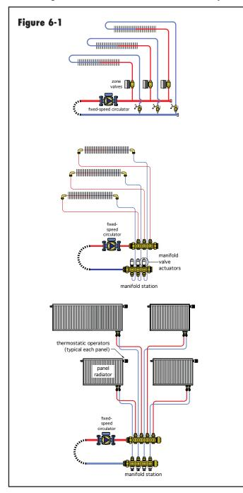
use electrically operated zone valves, and others use electrically operated manifold valve actuators connected to each internal valve within a manifold station. Still others use non-electric thermostatic radiator valves. All three types of systems are shown in Figure 6-1.
