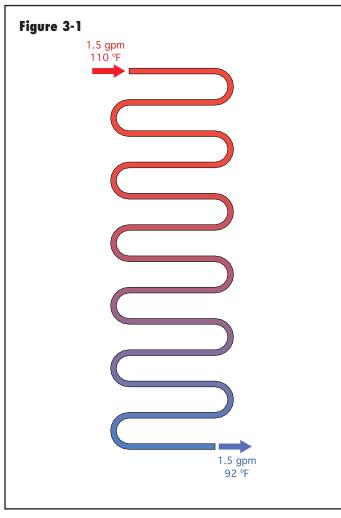
Solution: Using Formula 3-2, the rate of heat transfer from the circuit is:
