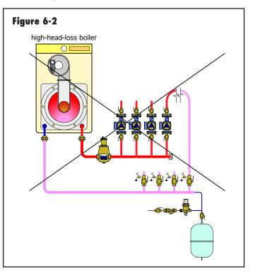
The high head loss of the mod/con boiler significantly increased the overall head loss of the common piping and largely negated the hydraulic separating characteristic attained in systems using the older style, low-headloss boilers. This created many problem installations, since installers and manufacturers did not immediately recognize the source of the resulting flow problems.
