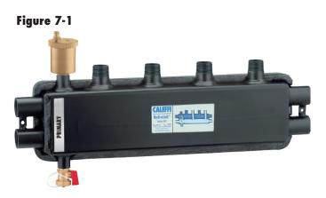
The HydroLink provides a chamber to hydraulically separate the boiler circuit from the distribution circuits. It also provides a self-contained manifold station that supplies up to four independently controlled load circuits with the same supply temperature. These features and their equivalent piping are shown in Figure 7-2.
