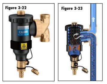
Figures 3-22 and 3-23 shows another variation on a magnetic dirt separator. In this case, the separator's body is made of engineered polymer. The body connects to a rotatable brass base fixture that allows the body to remain vertical regardless of the orientation of the pipe to which it is attached. This separator also contains a media that helps separate dirt from the flow stream. The magnetic collar can be seen at the lower end of the body.
