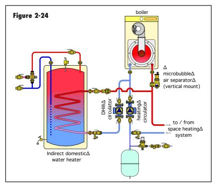
The surface on which microbubbles coalesce is called the "coalescing media." Some microbubble air separators use metal meshes for this media, while others use special polymers. In either case, the coalescing media must provide high surface contact area, enhancement of vertical bubble movement and a relatively low pressure drop.
