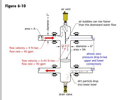
sufficient air collects at the top of the body, the float-type air vent allows it to be ejected from the system. Thus, a hydraulic separator can provide air separation.
