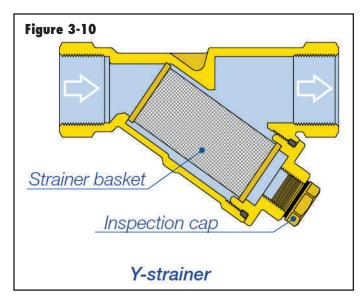
Y-strainers work similarly to the strainer inside the neck of a funnel. All system flow passes through the strainer and particles larger than the mesh size of the basket are trapped. Particles smaller than the mesh size may pass through the basket, as shown in Figure 3-11.
