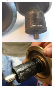
rotor can, preventing the circulator from operating.
