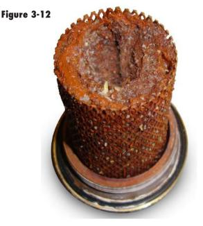
Flow reductions due to dirt accumulation in Y-strainers will reduce heat conveyance by the system. When restricted strainers are present near the inlet of circulators, they can induce vapor cavitation due to significant pressure drop. This can severely damage a circulator if not corrected.
