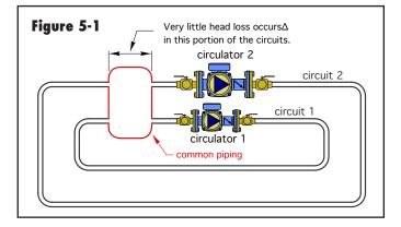
The degree to which two or more operating circulators interact with each other depends on the head loss within the piping path they have in common. This piping path is called the **common piping**, since it is shared by both circuits. The lower the head loss of the common piping, the less the circulators will interfere with each other.
