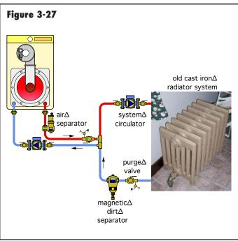
as shown in Figure 3-26. This is especially important in systems using boilers or other heat sources with compact heat exchangers. It's also very important in systems where a new boiler is installed in a system containing older piping and/or cast iron radiators, as shown in Figure 3-27.
