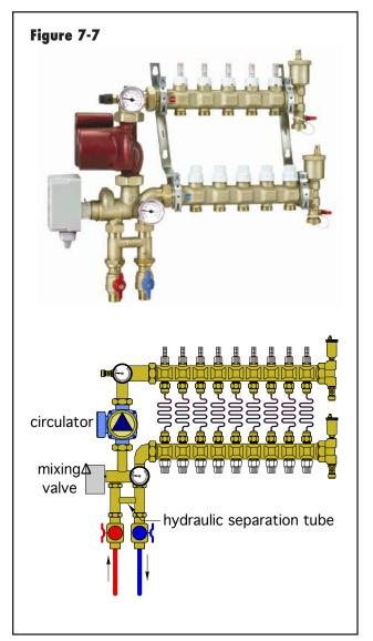
Caleffi also offers distribution manifold stations with integrated hydraulic separation details, an example of which is shown in Figure 7-7.
