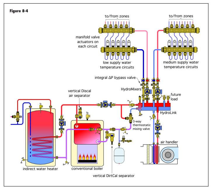
the manifold station as the manifold valve actuators open and close in response to zone thermostats. The supply water temperature from each HydroMixer can be independently adjusted. The mixing can be done with either a thermostatic valve or motorized 3-way valve.
