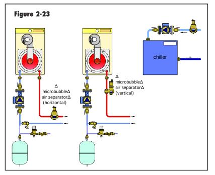
As microbubbles coalesce together, they form larger bubbles. Eventually, the bubbles attain a volume large enough that buoyancy forces overcome the adhesion forces holding them to the coalescing surface. The bubbles then rise along the coalescing surfaces to a chamber above the main flow stream where they can be collected and expelled through a float-type air vent. The concept of coalescence inside such a separator is illustrated in Figure 2-22b.
