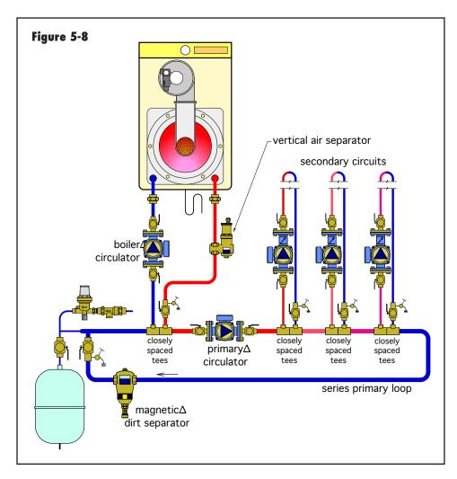
the secondary circulator operates. Because the flow created by the primary circulator does not induce flow in the secondary circuit, nor does it have any significant effect on the flow in the secondary circuit when its secondary circulator is operating, these two circuits are hydraulically separated from each other.
