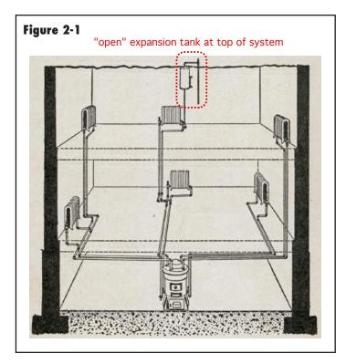
system—usually in the attic or upper floor, as seen in Figure 2-1, which appeared in a heating design manual published in 1906.
