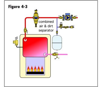
Combined air & dirt separators use the same principles of microbubble air separation in the upper portion of the separator body, combined with low-velocity-zone dirt separation in the lower portion of the separator body. They have a float-type
