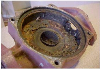
If oxygen continues to be present in the system, magnetite will be converted to hematite ( $Fe_2O_3$ ), which can cause pitting corrosion throughout the system.
