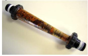
With sufficient accumulation, dirt buildup can cause the moveable parts in the flow meter to jam, rendering the meter useless.
