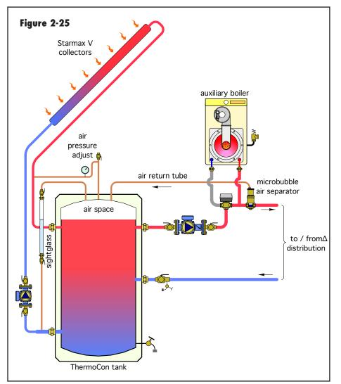
Also note that there is no expansion tank in this system. The captive air volume at the top of the storage tank, if properly sized, provides the volume needed to accommodate the expansion volume of the system's water and serve as the drainback space.
