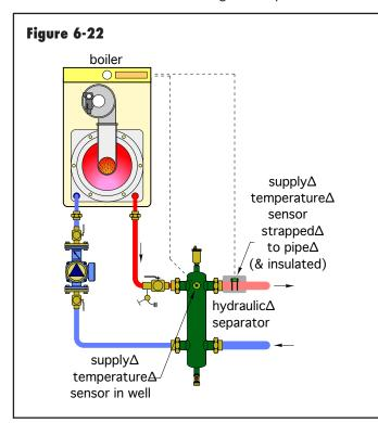
**Case #3: Distribution system flow is less than boiler flow:** Again, since the flow rates on opposite sides of the hydraulic separator are not equal, mixing will occur inside the separator. In this case, a portion of the hot water entering from the boiler circuit moves downward through the separator and mixes with cool water entering from the distribution system, as shown in Figure 6-23.
