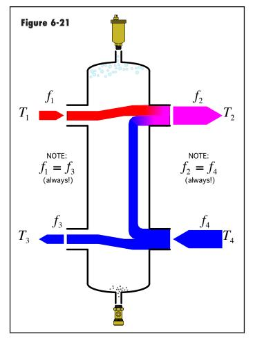
returning to the heat source from port 3 equals the temperature returning from the distribution system into port 4. Again, very little mixing takes place within the separator. Dirt particles carried into the separator at port 4 will settle to the bottom of its body, where they can be periodically flushed out through the drain valve.
