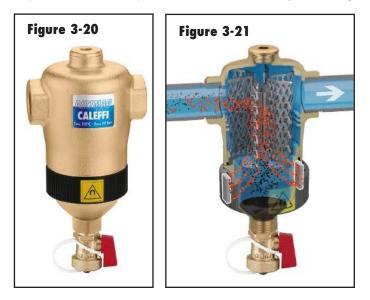
powerful rare-earth magnets on or within the separator. Iron oxide particles are attracted to these magnets, improving the capture efficiency of the separator. When the magnetic portion of the separator is removed, the iron oxide particles along with other debris can be flushed out from the lower bowl of the separator.
