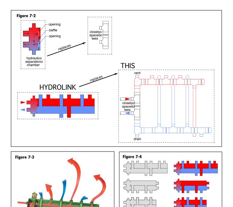
A typical configuration for the HydroLink has the heat source connected to the "primary" chamber piping on the left side of the unit, along with several load circuits connected to the other "secondary" connections that connect into the manifold chamber. Two additional tapped connections are provided in the top and bottom of the primary chamber for mounting an air vent and drain valve/makeup water assembly, as shown in Figure 7-5.
