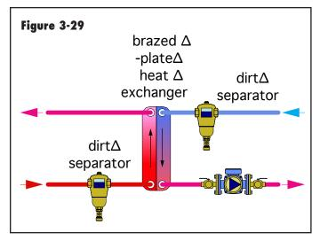
In systems with a main mixing valve, it's best to place dirt separators in the return line from the distribution system ahead of the valve. This increases flow through the separator and better protects the mixing valve from dirt.
