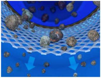
As debris collects inside the strainer's basket, it impedes flow. This results in increased pressure drop and hence higher head loss. If the strainer basket is not properly maintained, such head loss can be excessive. Figure 3-12 shows an example of a heavily loaded basket from a Y-strainer.
