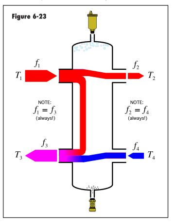
This condition occurs when the boiler heat output rate is (temporarily) higher than the current system load. Under this condition, heat is being injected into the system faster than the load is removing heat. This produces a relatively fast increase in boiler return temperature. If a modulating boiler is being used, this will lead to a relatively fast decrease in firing rate, which usually will result in a reduction in boiler-side flow rate.
