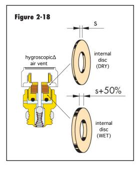
When the knob is fully closed, an internal O-ring seals off the side port. However, if air is present at the vent, the fiber discs will dry and allow air to pass through them. This air is discharged under the vent's knob, as shown in Figure 2-19b. Once the air has been vented and water reaches the fiber discs, they swell very quickly to seal off any further discharge.
