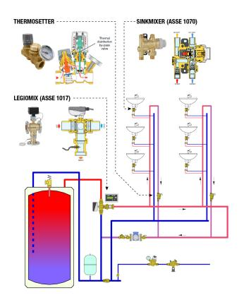
Rheem 120 gallon water heaters and one 120 gallon storage tank. For the domestic hot water (DHW) distribution, Performance Plumbing chose the full Caleffi LEGIOMIX® DHW control system (a 1.25 in. LEGIOMIX Station electronic point-of-distribution mixing valve, ThermoSetter<sup>TM</sup> thermal balancing valves and SinkMixer<sup>TM</sup> point-of-use mixing valves).
