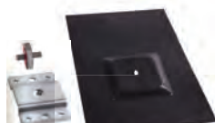
Flashing kit with 3/8" stud for attaching U mounts and other brackets using the supplied 3/8" stainless steel nut & washer. Black painted aluminum 6061 T6 flashing 14¾"L x 9½"W x 0.6"H, galvanized steel base plate with six mounting holes and double stud.
