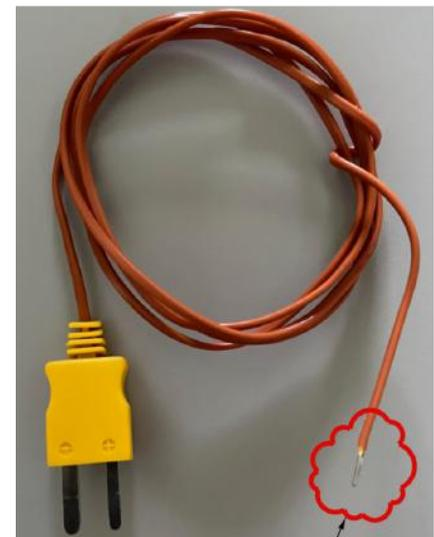
end of thermocouple that senses temperature
