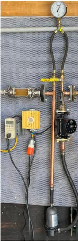
zone in the system, recording the flow rate produced within each zone by its associated zone circulator.
