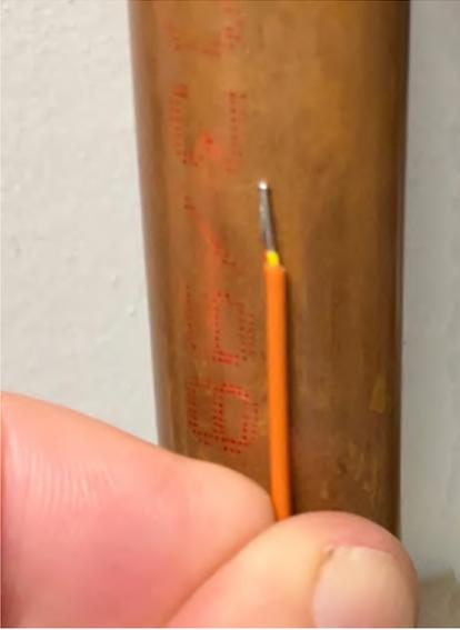
to measure a temperature difference in a hydronic circuit, they should both be mounted to pipe surfaces *using identical methods*.
