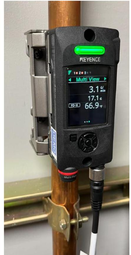
This meter can be quickly mounted to the outside of a pipe. It can be used with a wide range of pipe materials and sizes, as well as different fluids, and over a wide range of temperatures. Reported accuracy is +/-3% of the reading value. When equipped with optional platinum RTD temperature sensors, the meter shown in figure 3-8 can directly measure the  $\Delta T$  of a hydronic circuit and combine that measurement with flow rate to calculate the rate of heat transfer.
