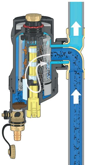
The filter mesh is characterised by various parameters, one the most important being the mesh size (or filtering capacity), which indicates the minimum dimensions of the particles that the filter is able to intercept. Another concerns the filter mesh surface, with a larger surface area guaranteeing a lower degree of fouling.
