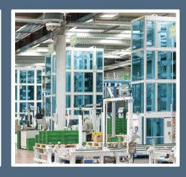
2. THE VERTICAL AUTOMATED WAREHOUSE IS COMPRISED OF FREE-STANDING METAL STRUCTURES COMPLETE WITH AUTOMATED HANDLING SYSTEMS.
