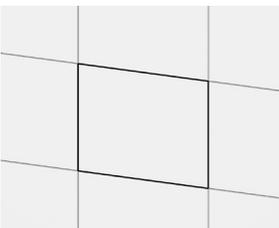
Plaster or tile the inspection port to achieve the same effect as used on the wall.
