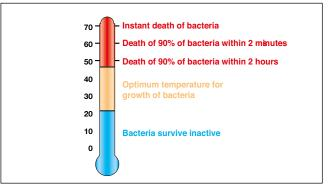
To ensure correct thermal disinfection, it is necessary to go up to values of at least  $60^{\circ}$ C.
