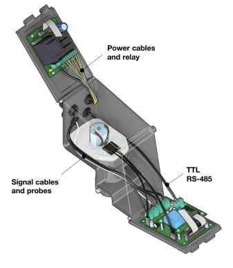
Connections layout: connections must not create thrust stresses on the circuit board.
