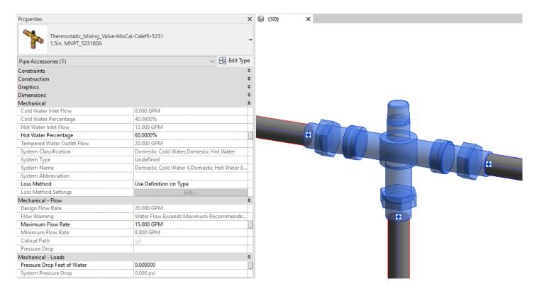
Figure 5 – The Caleffi 5231 MixCal Thermostatic Mixing Valve families can be found under pipe accessories in the project browser and placed directly onto pipe of the same size. It will then read flows and consider pressure drop in the system. In this case, it shows a message that the water flow exceeds the maximum allowable.
