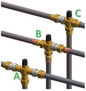
Figure 3 - Caleffi 5231 MixCal Thermostatic Mixing Valve
