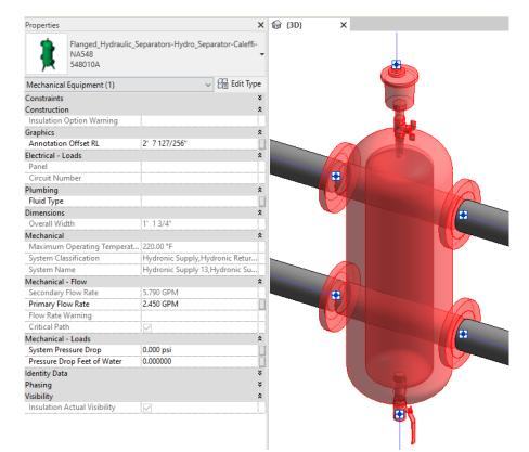
Figure 5 – The OBCaleffi 548 and NA548 Series Flanged Hydraulic Separator families can be found under pipe accessories in the project browser and placed directly onto pipe of the same size. It will then read flows and consider pressure drop in the system.
