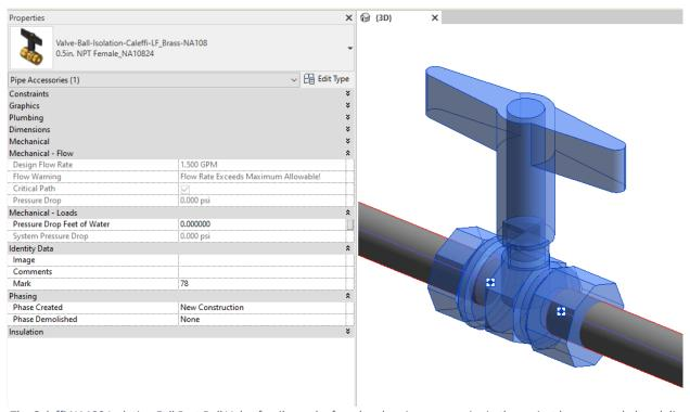
Figure 5 – The Caleffi NA108 Isolation Full Port Ball Valve family can be found under pipe accessories in the project browser and placed directly onto pipe of the same size. It will then read flows and consider pressure drop in the system.
