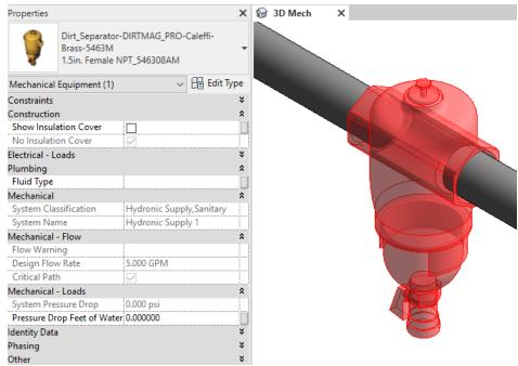
Figure 5 – The 5463M DIRTMAG Pro family can be found under pipe accessories in the project browser and placed directly onto pipe of the same size. It will then read flows and consider pressure drop in the system.
