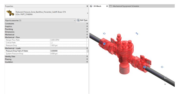
Figure 5 – The Caleffi 574 RPZ Backflow Preventer family can be found under pipe accessories in the project browser and placed directly onto pipe of the same size. It will then read flows and consider pressure drop in the system.
