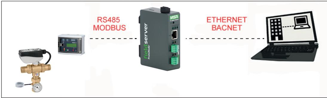
Connect a CAT5 Ethernet cable (Straight through or Cross-Over) between the local PC and gateway.
