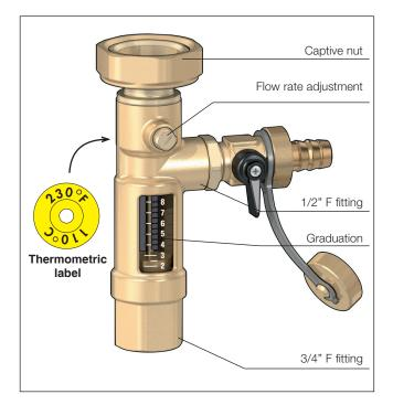
A thermometric label on the back of the flow meter signals if the maximum permitted temperature (230°F/110°C) has been exceeded: white = temperature not exceeded;
