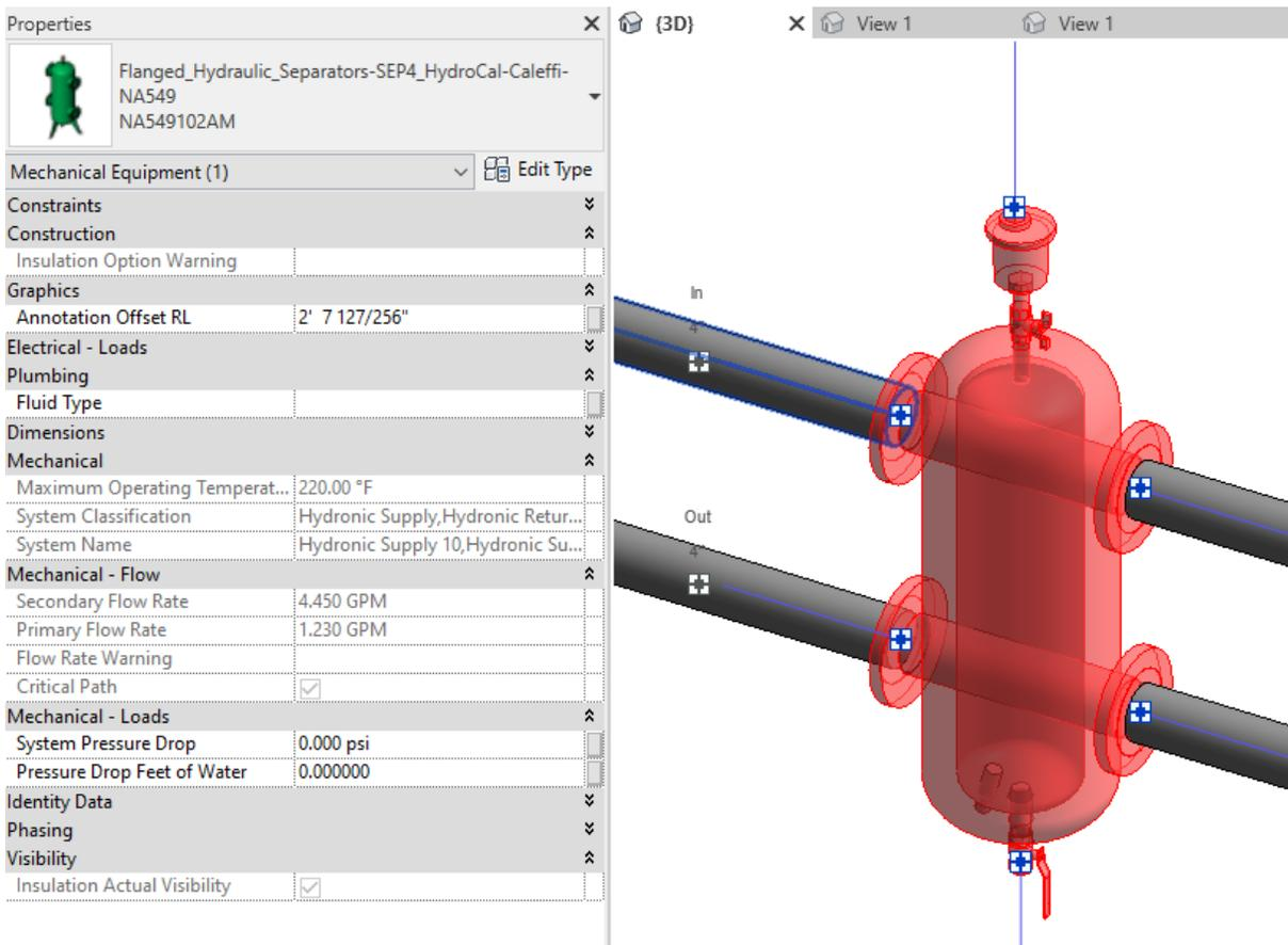
Figure 5 – The OBCaleffi SEP4™ 549 and NA549 Series Flanged Hydraulic Separator families can be found under pipe accessories in the project browser and placed directly onto pipe of the same size. It will then read flows and consider pressure drop in the system.
