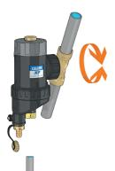
The Caleffi XF magnetic filter is adjustable so that it can be installed on both horizontal and vertical pipes. Use the special tightening wrench to screw and unscrew the locking nut. The functional and fluid-dynamic characteristics remain unchanged in both configurations.
