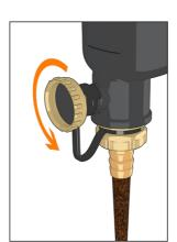
3. Turn the top knob clockwise to clean the filter mesh with the special internal brushes. Turn a few times to clean properly.
