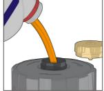
Liquid additives can only be added if shut-off valves have been installed downstream and upstream of the device.
