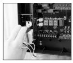
Slide bottom end of transformer into bottom latch.
