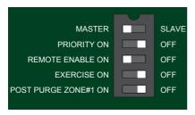
The ZSR series of control is programmed by positioning five dip switches for the following operations.
