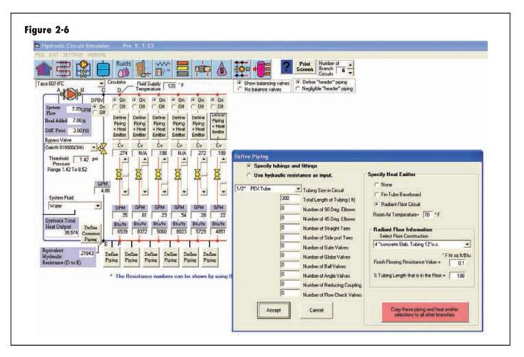
Figure 2-6 shows a screen from one software program that can simulate the thermal and hydraulic behavior of a multiple crossover hydronic system, including the effect of balancing valves and a differential pressure bypass valve.
