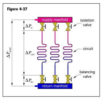
This diagram labels the pressure drop between the supply and return manifolds as  $\Delta P_{total}$ . This circuit with the highest pressure drop is found by combining the largest of the three circuit pressure drops ( $\Delta P_{circuit}$ ) with the pressure drop through a fully open isolation valve ( $\Delta P_{iv}$ ), plus the pressure drop through a fully open balancing valve ( $\Delta P_{bv}$ ). This relationship is expressed as Formula 4-8.
