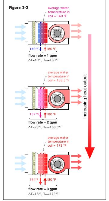
As the flow rate through the coil increases, the temperature difference between its inlet and outlet decreases. This means that the average water temperature in the coil increases, and so does its heat output. This holds true for all other hydronic heat emitters, such as radiant panel circuits, panel radiators and baseboard.
