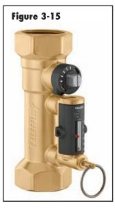
The meter scale on the front of this valve is fully isolated from the system's fluid. The flow indicator on the scale is moved by the force created by a magnetized element within the bypass chamber behind the meter scale. This prevents discolored fluid or particulates in the flow stream from distorting the meter scale.
