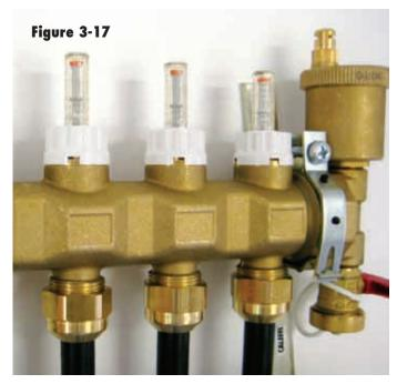
across the precision orifice in the main flow passage. As the spring-loaded assembly moves, magnetic forces move the indicator on the meter scale. When the ring is released, flow through the bypass chamber stops. This valve, which can be mounted in any position, also allows adjustment of flow rate by turning the stem located above the flow meter.
