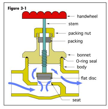
Globe valves should always be installed such that flow enters the lower body chamber, and moves upward toward the gap between the seat and disc. This allows the disc to close against the area of higher pressure. Reverse flow through this type of valve can cause unstable flow regulation, cavitation, and noise. All globe valves have an arrow on their body indicating the proper flow direction.
