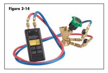
In the past, the differential pressure across the balancing valve's ports was measured with relatively simple devices, such as manometer, or accurate differential pressure gauge. Modern instruments use electronic pressure transducers and the necessary electronics to convert the measured differential pressure directly to flow rate. The flow rate is then displayed on the handheld device. Such devices can cost several hundred dollars, depending on capabilities.
