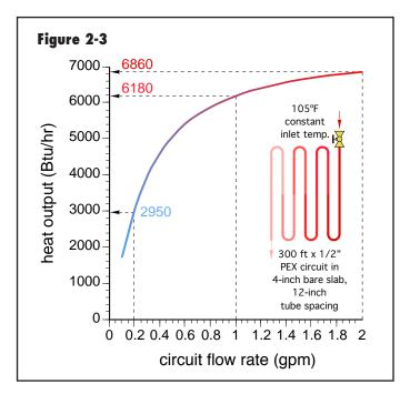
This floor heating circuit's maximum heat output of 6,860 Btu/hr occurs at the maximum flow rate shown, (2.0 gpm). Decreasing the circuit's flow rate by 50% to 1.0 gpm decreases its heat output to 6,180 Btu/hr, a drop of only about 10%. Reducing the flow rate to 10% of the maximum value (0.2 gpm) still allows the circuit to release 2,950 Btu/hr, about 43% of its maximum output.
