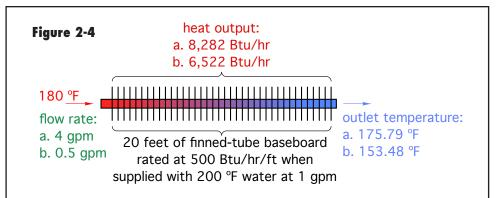
The outlet temperature of the baseboard can be determined using Formula 2-1:
