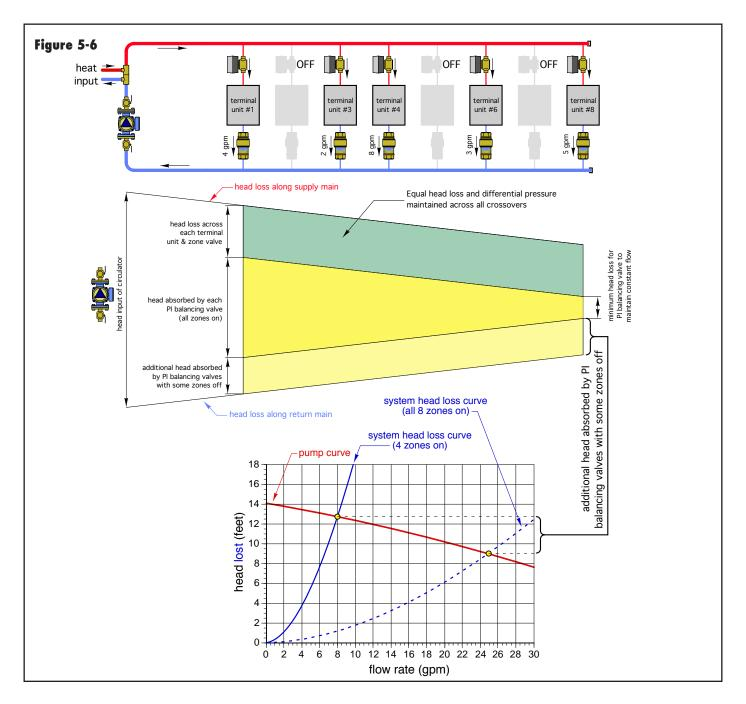
added to the system when a variable-speed pressure-regulated circulator is used.
