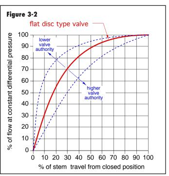
Notice that when the valve's stem reaches the 50% open position, the valve is passing approximately 90% of the flow it will pass when fully open.
