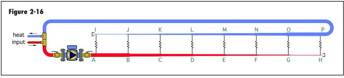
• The higher the ratio of the head loss through the crossovers divided by the head loss through the mains, the closer the reverse return system will be to "self-balancing" (e.g., equal flow rates in all crossovers).
