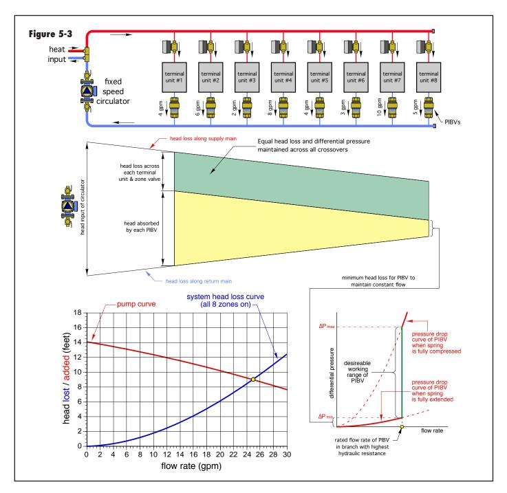
This head loss could also be estimated by assuming a typical mains piping sizing criteria of 3 to 5 feet of head loss per hundred feet of pipe.
