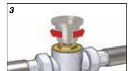
Temperature adjustment cap in place
