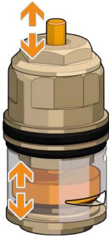
10. Doing so rotates the shutter as required by the maximum flow rate. A table that shows how to select the setting number is provided later in this section. This adjustment does not affect the stroke of the stem, only the size of the flow aperture when the valve is fully open. This is an important feature because the proportional control signal to the valve's actuator is always fully utilized for the full stroke of the shaft, even when the maximum flow rate through the valve is reduced.
