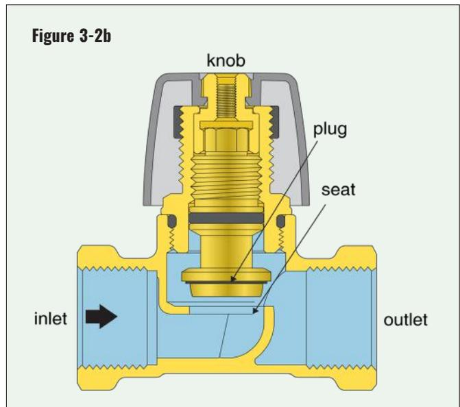
upstream chamber in the valve, and the other connects to the downstream chamber. The differential pressure is measured across the orifice between these chambers. The knob on the valve controls the position of the valve's plug relative to the seat, and thus, the size of the orifice (e.g., the "gap" between the plug and the seat). Hence the designation "variable orifice."
