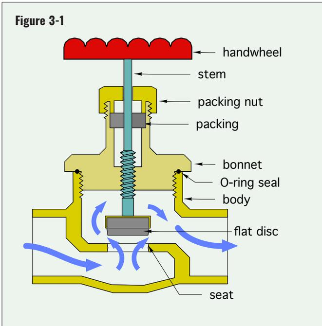
The simplest type of balancing valve is a globe valve, a cross section of which is shown in figure 3-1.
