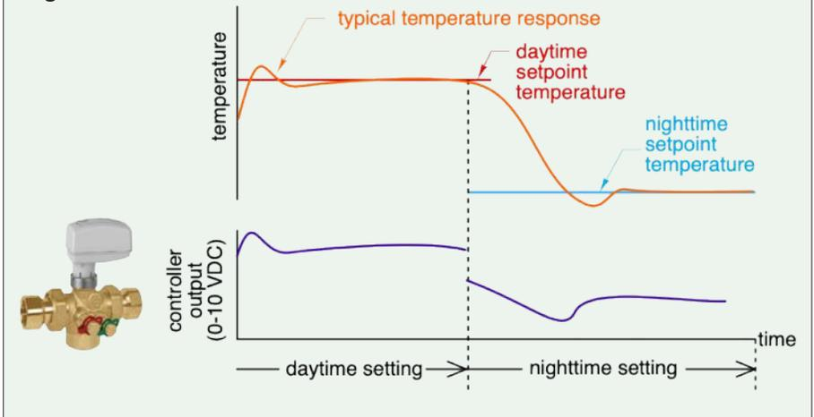
to quickly stabilize room temperature at the desired setpoint with very minimal overshoot or undershoot, as represented in figure 5-7.
