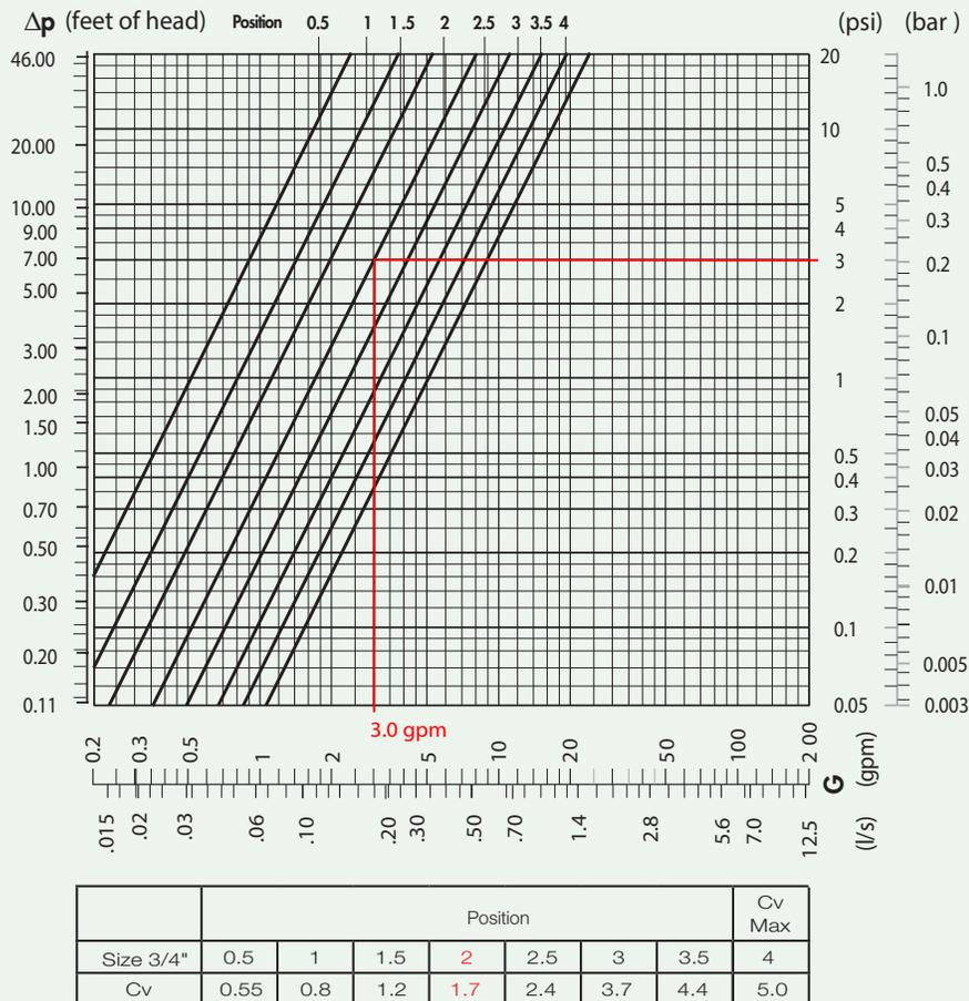
**BALANCING VALVES WITH FLOW INDICATION**
