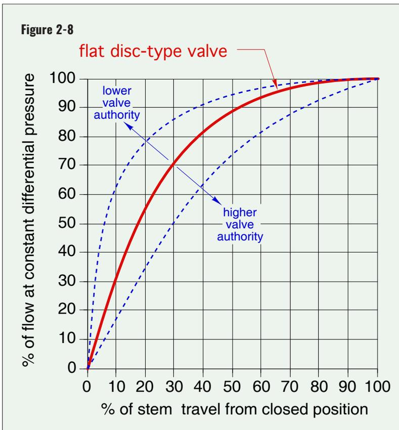
Figure 2-8 shows how valve authority affects the relationship between the stem position of a globe valve and the percentage of flow passing through the valve.
