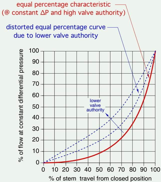
A distorted equal percentage characteristic, although not ideal, is still preferable to a quick-opening characteristic when the valve is used to regulate the heat output of a heat emitter. The overall effect will be a heat output characteristic versus valve stem position curve that is not linear. Heat transfer will increase slightly faster at low flow rates.
