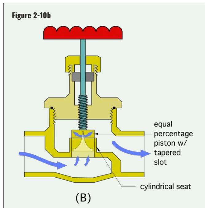
emitter being controlled, designers have created valves with different internal “trim.” One of the most common trims gives a valve an “equal percentage characteristic.” Flow through this type of valve increases exponentially with upward movement of the stem.
