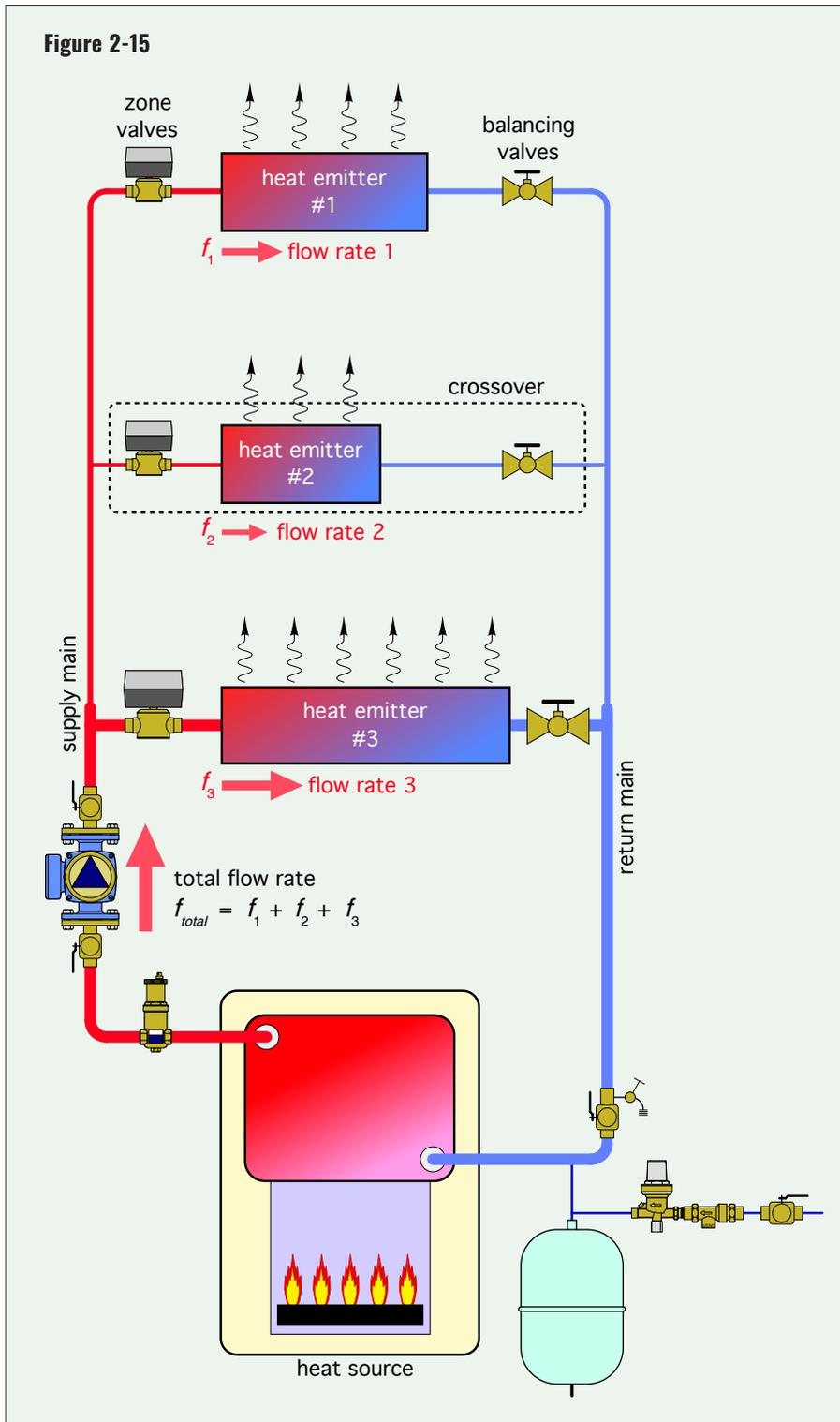
It's possible to calculate the flow rates that will occur in any of the branches based on the status of the zone valves and the settings of the balancing valves. However, those calculations can be complex, especially for larger systems with many branches. Such calculations are typically done using computer models of the piping system.
