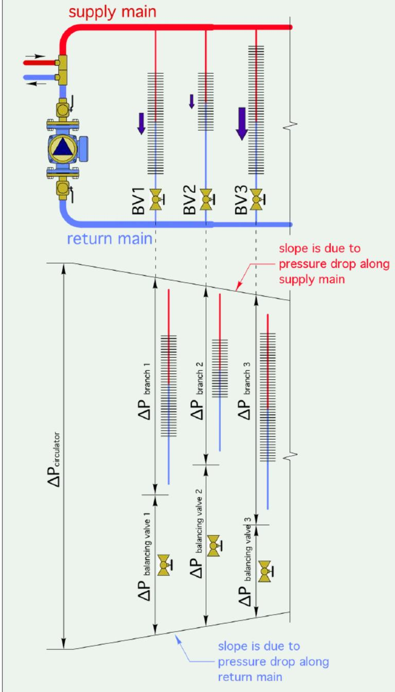
assumed to be sized so that it can provide the necessary differential to drive flow through the least-favored branch, accounting for the head loss along the full length of the supply and return mains.
