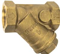
The NA109 series low-lead brass y-strainers are designed for residential and commercial plumbing and hydronic applications to protect equipment from premature failure due to damaging debris. Y-strainers are used to protect critical water control devices such as backflow preventers, pressure reducing valves, balancing valves and control valves. The NA109 series are available with 1/2" to 2" FNPT connections and have a 30 mesh stainless steel screen.
