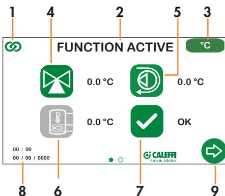
1. **Caleffi Cloud symbol:** this appears in colour when the device is connected to the Caleffi Cloud, and in grey when not connected;
