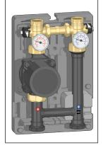
In versions with a EVOSTA2 pump, the electronic part of the pump must be rotated by unscrewing the four screws, as indicated by the arrows, and turning the body clockwise by 180°. If this step is not performed, it will not be possible to fit the unit back inside the insulation.
