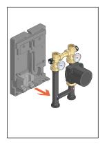
In versions with a UPML 25-105 pump, the electronic part of the pump must be rotated by unscrewing the four screws, as indicated by the arrows, and turning the body anticlockwise by 90°. If this step is not performed, it will not be possible to fit the unit back inside the insulation. In A2L versions with a UPM3 Auto L pump, no changes to the circulators are required.
