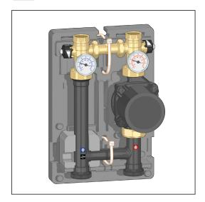
When fitting the rear shell to the assembly, it is recommended to use two clamps, as shown in the figure, to ensure that the insulation adheres perfectly to the pipes and to minimise the likelihood of condensation build-up.
