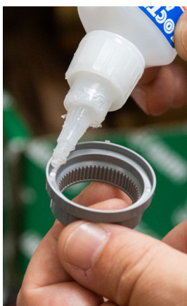
18 - Apply four dots of glue to the locking nut
