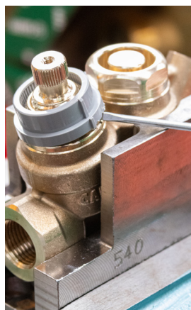
3 - Remove the plastic locking nut using a screwdriver (NOTE: the locking nut is glued to the body)
