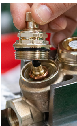
15 - Put the headwork back in position
