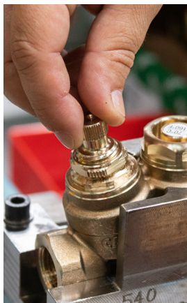
17 - Fully loosen the knob holder to reach the maximum temperature position
