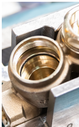
11 - Position the O-ring back in its seat
