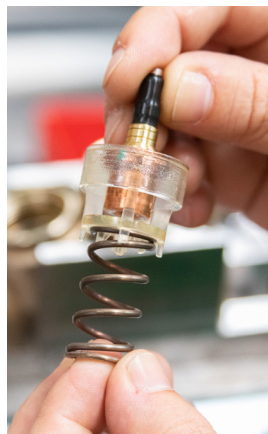
13 - Assemble the sensor, obturator and spring
