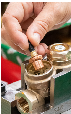
6 - Remove the sensor
