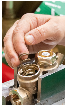
8 - Remove the spring
