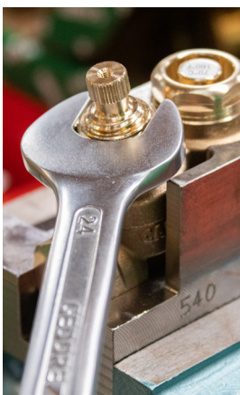
4 - Unscrew the headwork
