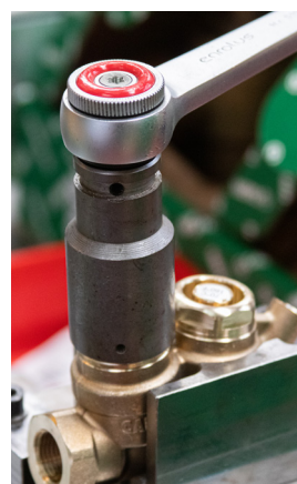
16 - Screw on the headwork. Tightening torque 15–20 N•m
