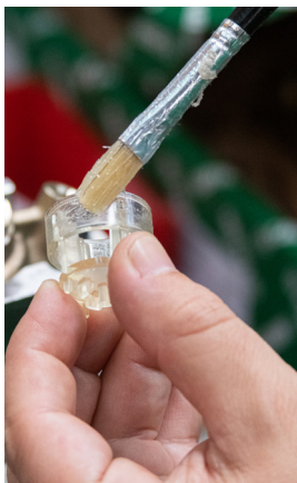
12 - Grease the obturator
