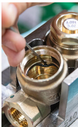
9 - Remove the O-ring from its seat. (NOTE: only if the O-ring is damaged)
