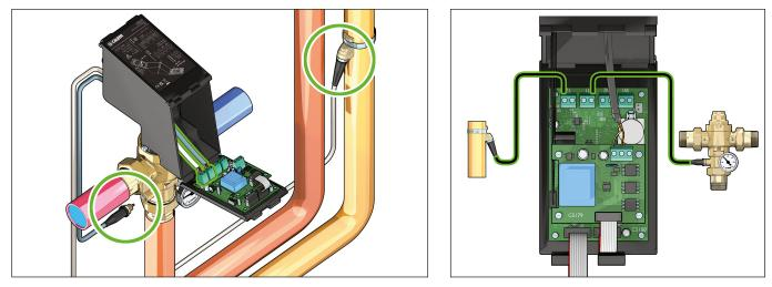
Perform the hydraulic installation of the temperature probes and provide electrical wiring.
