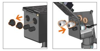
Connections layout: connections must not create thrust stresses on the circuit board.
