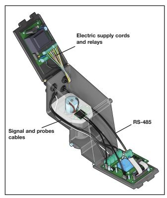
If it becomes necessary to use the top cable glands, remove the grommets and insert the cable glands
