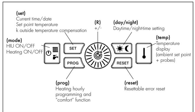
The digits in the center of the display show the current ambient temperature, if the thermostat function is enabled. In case the latter is disabled, the digits show DHW temperature and heating flow temperature when the HIU is in operation, "--." when in stand-by.
