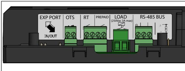
All the terminals are mounted on removable connectors to facilitate wiring operations.
