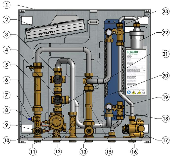
**Characteristic components SATK2240. (HIGH temperature with pump)**
