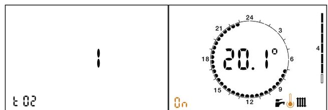
The circulator has to be fed through the auxiliary microswitch so that the control of recirculation is carried out by the heat interface unit. DHW recirculation (t02=1) disables the other functions operating on the auxiliary microswitch described on page 16. Refer to page 16 for the electrical characteristics of the microswitch.
