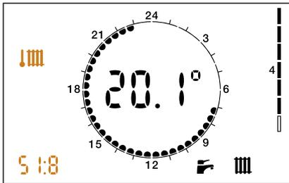
**Heating flow probe temperature (SATK2210. - SATK2220.)**
