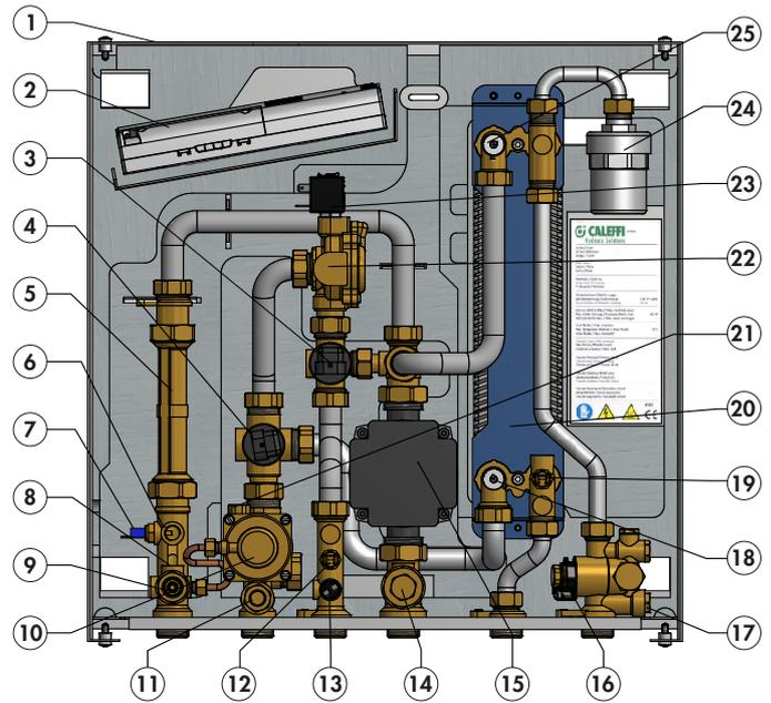
**Characteristic components SATK2220. (MEDIUM temperature)**
