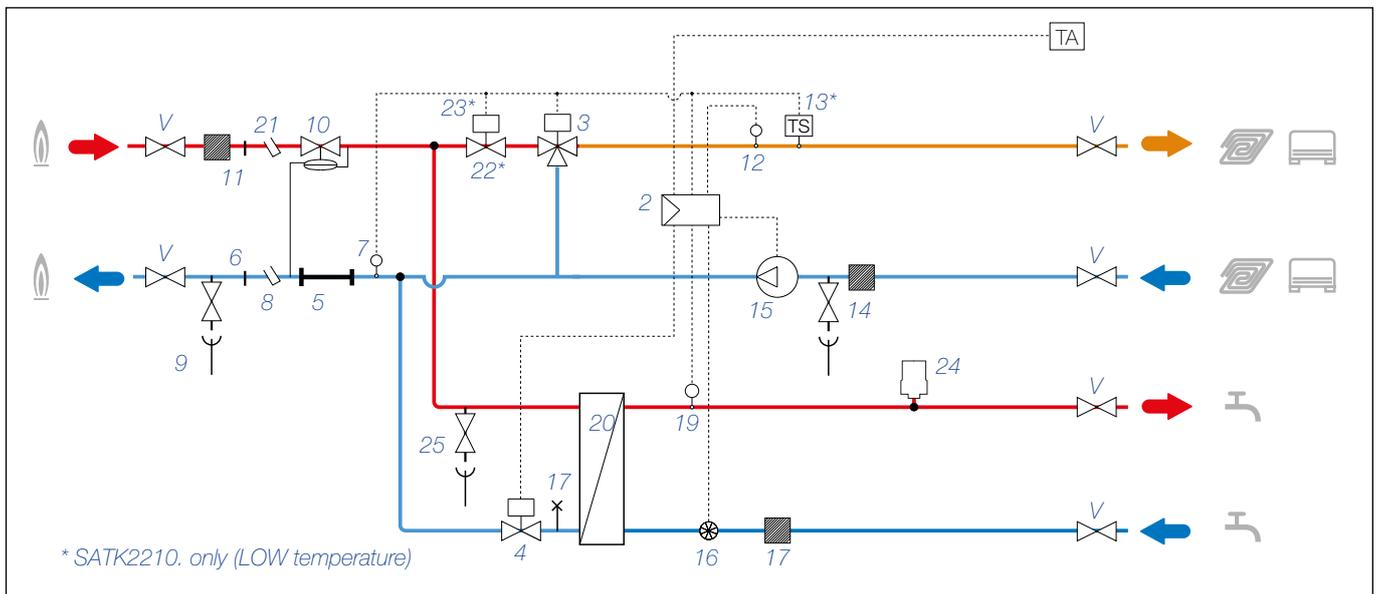
**Characteristic components SATK2230. (HIGH temperature)**
