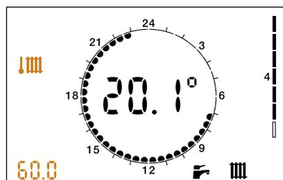
Heating flow temperature (SATK2210. - SATK2220.)
