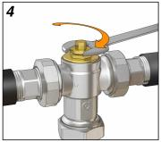
Lock adjustment spindle with locking nut
