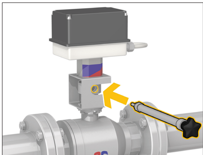
2) Screw the specific lever (supplied) into the locking pin hole.
