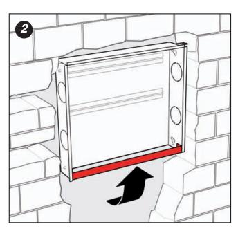
After assembling the manifolds in the box, use the supplied cardboard sheet to protect the box when completing the walling in. To use the sheet, rest the "L" fold on the top of the box, with the other end resting on the edge of the galvanized bar.
