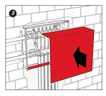
After removing the cardboard sheet and galvanized bar, refit the false frame by screwing in the four butterfly screws inside the box and then replace the cover.
