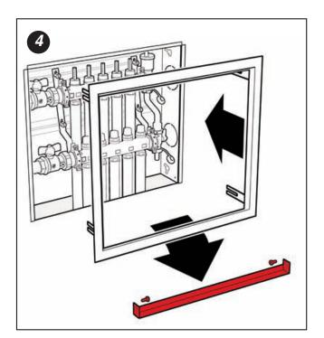
NB: The parts in red are used during fitting and finishing and then discarded.
