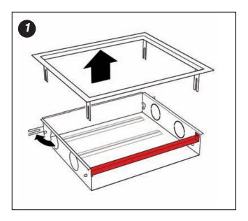
Rotate the galvanized bar so that it matches the surface of the outside walls as shown.
