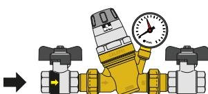
**IMPORTANT:** The installation must be performed with the BALLSTOP valve upstream and respecting the flow direction indicated by the arrows.
