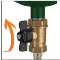
To purge the ferrous impurities in the steel DIRTMAG, the flexible magnetic stack is removed from the brass dry-well and, with the system still running, the drain valve is opened. Aided by the system pressure, the dirt and ferrous impurities, including magnetite flushes out quickly and effectively.
