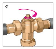
Lock adjustment spindle with locking nut
