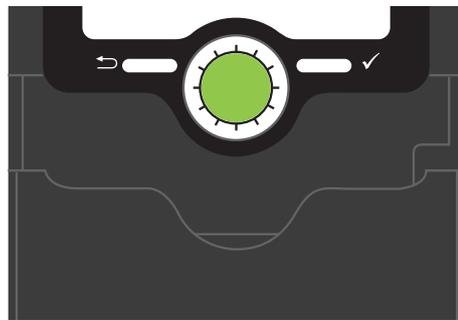
The controller is operated via 2 buttons and 1 adjustment dial (Lightwheel®) below the display:
