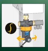
When necessary, it is possible to use the cap with a manual air vent to eliminate air inside the strainer.
