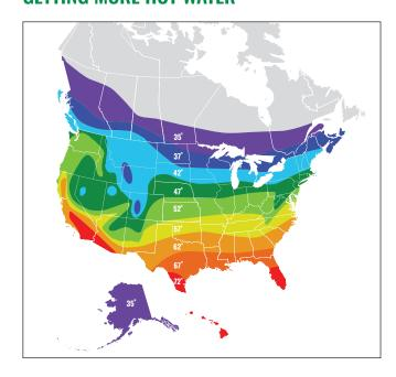
Determine your ground water temperature from this map. This is the supply water temperature to your water heater.
