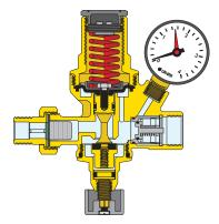
Regulation is performed by means of the regulator inside the top cover; turning the regulator clockwise or anti-clockwise respectively increases or decreases the pressure at which the unit operates.
