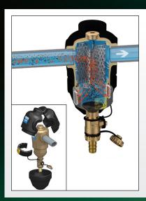
Magnetic dirt separators are based on the principle of collision against the mesh and particle decantation, making them more effective than common strainers.
