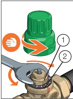
Turning the locking nut (1), which determines the number associated with the "Adjustment position", results in opening/closing of the bore cross section in the external obturator (4). Hence, each bore cross section set on the locking nut corresponds to a specific  $G_{max_x}$  value.
