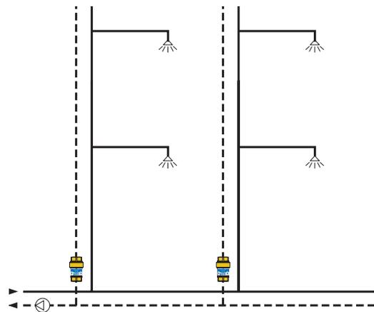
To adjust the flow rate to each riser or secondary branch of a system
