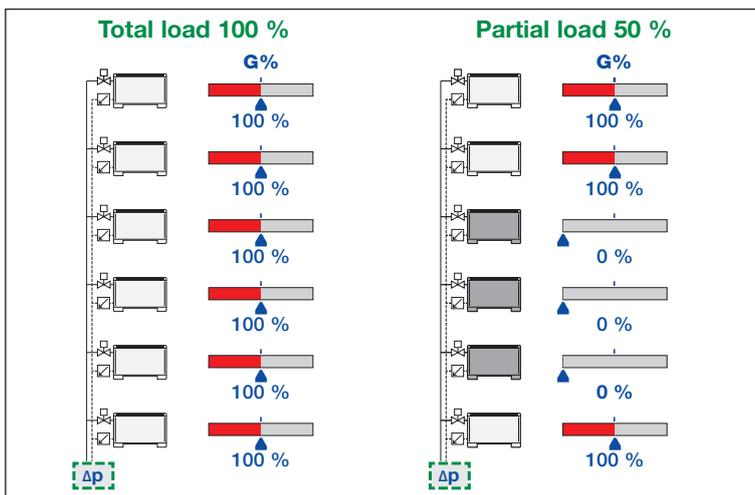
Dynamic devices can balance the hydraulic system automatically, ensuring each terminal receives the design flow rate. Even when the regulating valves close the circuit partially, the flow rates in the open circuits **remain constant at the nominal value.** The system always guarantees the greatest comfort and the highest energy savings.
