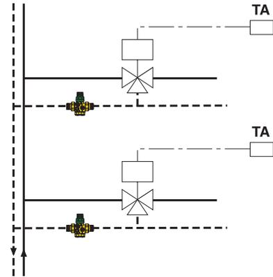
To adjust flow rate in applications with cooling beams
