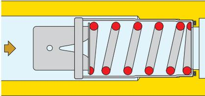
If the differential pressure is within the control range, the piston compresses the spring and gives the medium a free flow area to permit normal flow at the **nominal flow rate** for which the AUTOFLOW® is set.
