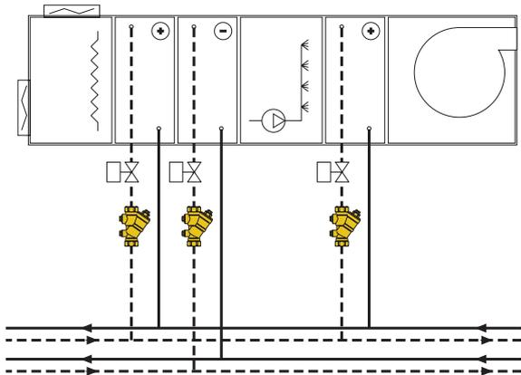
To balance the circuits that serve chiller unit evaporators or condensers
