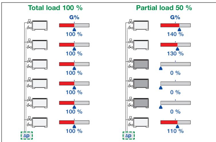
Traditionally, hydraulic circuits are balanced using manual setting valves. With these static devices, these circuits are difficult to balance perfectly and have **operating limitations** in the event of partial closure by means of the regulating valves. The flow rate in the open circuits **does not remain constant at the nominal value.**
