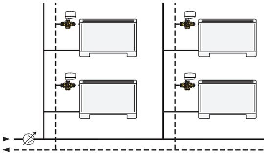
To balance circuits that serve air handling units
