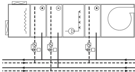
To guarantee the design flow rates (with open or closed valve) to the various zones of a system
