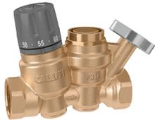
Thermostatic regulator for domestic hot water recirculation circuits. Complete with automatic thermostatic thermal disinfection function. With temperature gauge for circuit temperature checking. **“LOW LEAD”** dezincification resistant alloy body **CR**.
