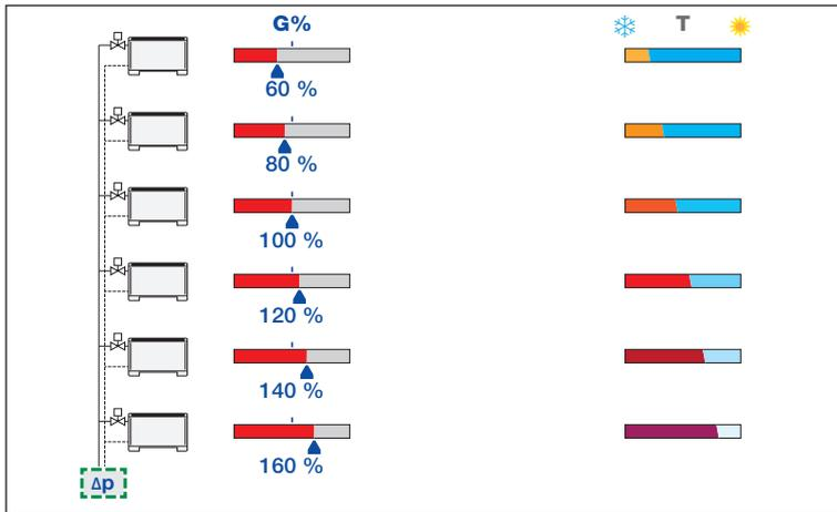
In unbalanced circuits, the hydraulic imbalance between terminals creates areas with non-uniform temperatures, resulting in problems with thermal comfort and higher energy consumption.
