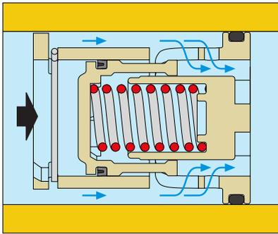
If the differential pressure is within the control range, the piston compresses the spring and gives the medium a free flow area to permit normal flow at the **nominal flow rate** for which the AUTOFLOW® is set.
