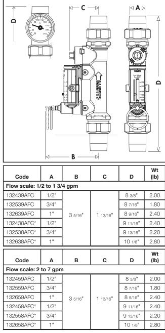
\*with dual-scale temperature gauge 30 - 210°F (0 - 100°C).
