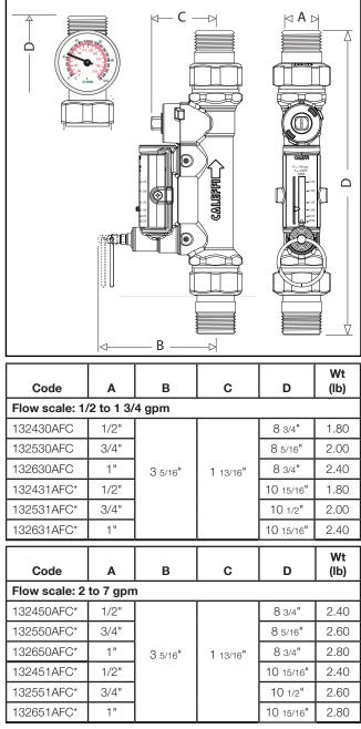
\*with dual-scale temperature gauge 32 - 210 °F (0 - 100 °C).
