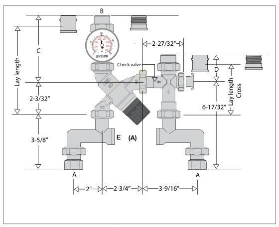
(A) This kit provides one pivot connector with a 3/4" FNPT port (E), which can be used for applications where there is no pressure relief valve on the tank. Install that pivot connector on the hot side to add a pressure relief valve. For applications where a pressure relief valve is present on the tank, install the pivot connector with the FNPT port on the cold side for incorporating an expansion tank.
