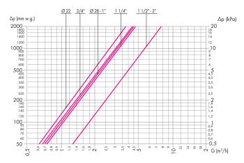
The maximum recommended medium flow speed to the device connections is  $\sim$  1,2 m/s.
