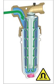
The water passes through the centre of the cartridge and comes into contact with the internal elements (Cu alloy -Zn/Ti), where the battery effect and whirling motion cause the first aragonite crystals to form.
