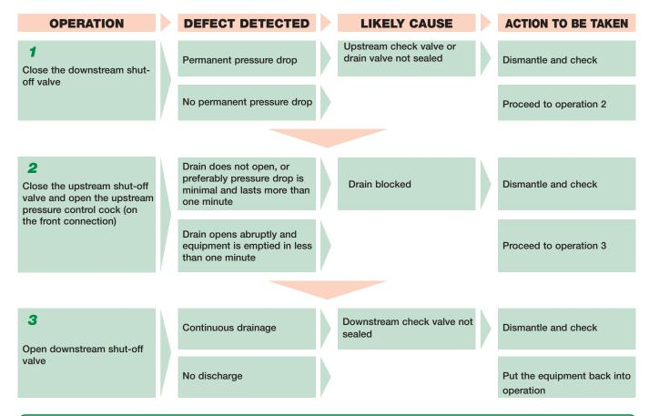
N.B.: In normal operation the appliance must not present any permanent pressure drop. Otherwise dismantle and verify.
