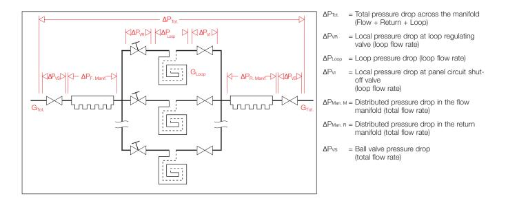
$\Delta \mathbf{P}_{\text{Tot.}} = \Delta \mathbf{P}_{\text{VR}} + \Delta \mathbf{P}_{\text{Loop}} + \Delta \mathbf{P}_{\text{VI}} + \Delta \mathbf{P}_{\text{Man. M}} + \Delta \mathbf{P}_{\text{Man. R}} + \Delta \mathbf{P}_{\text{VS}} \times \mathbf{2}$ (1.1)
