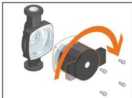
In versions with a UPML 25-105 pump, the electronic part of the pump must be rotated by unscrewing the four screws, as indicated by the arrows, and turning the body anticlockwise by 90°. If this step is not performed, it will not be possible to fit the unit back inside the insulation. In A2L versions with a UPM3 Auto L pump, no changes to the circulators are required.
