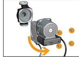
5. Assemble the unit as shown in the figure and fully tightening the captive nuts, taking care to position the seals correctly.
